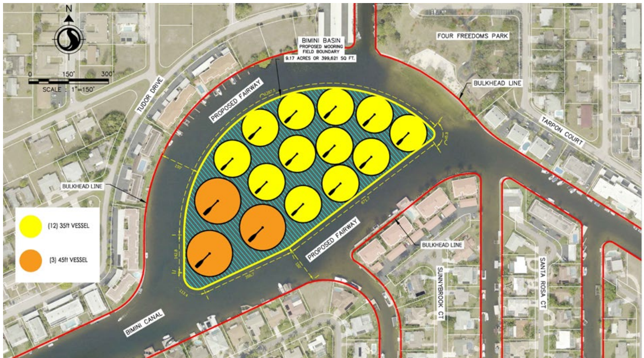
Figure 4: Option 2 - Proposed Mooring Field Layout with Moorings for Vessels up to 35 Feet (12) and 45 (3) Feet in Overall Length
