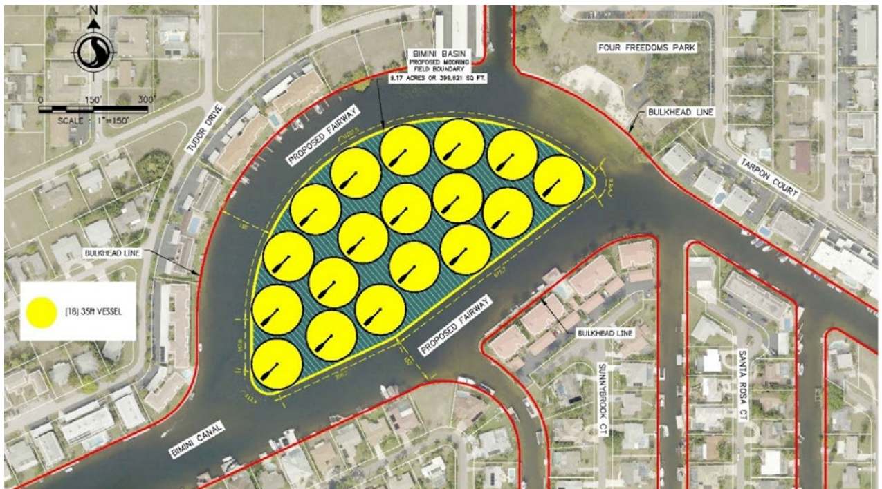
Figure 3: Option 1 - Proposed Mooring Field Layout with Moorings for Vessels up to 35 Feet in Overall Length
